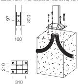
\*Element calculated for type II terrain and 29m/s wind, with soil made up of loose or wet sand of medium compactness (E0= 4800 kN/m²) and HM-20 concrete foundation. We offer adaptations for more demanding types of terrain and climatic conditions.
